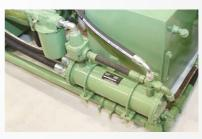
All MSG TURBO-AIR compressors feature a self-contained, low-pressure lubrication system.
